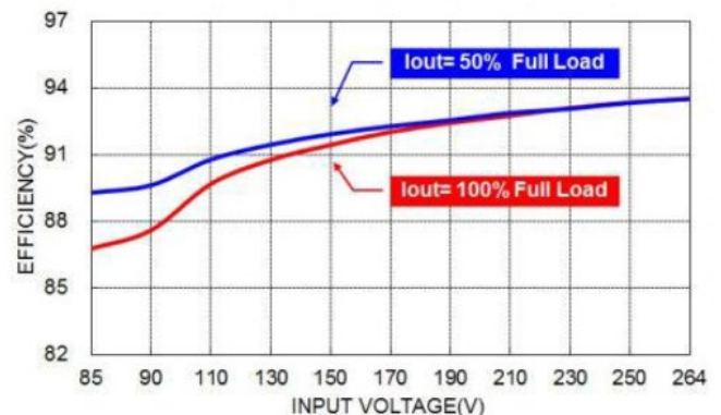
PSESL500-24S Efficiency vs. Input Voltage
