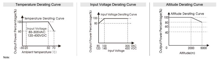
1. With an AC input voltage between 85-100VAC and a DC input between 120-140VDC the output power must be derated as per the temperature derating curves. 2. This product is suitable for applications using natural air cooling: for applications in closed environment, please contact factory.
