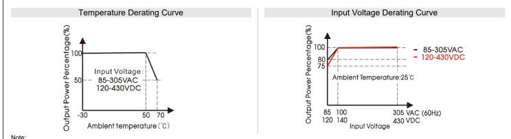
1. With an AC input voltage between 85-100VAC and a DC input between 120-140VDC the output power must be derated as per the temperature derating curves. 2. This product is suitable for applications using forced air cooling: for applications in closed environment, please contact factory.
