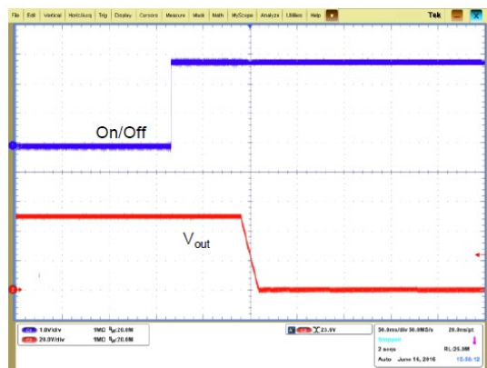
Shutdown from On/Off, Vin=220VAC, 100% Load
