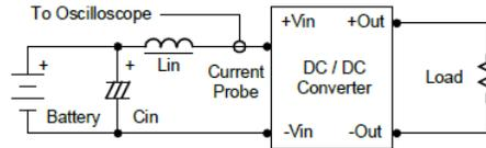
Peak-to-Peak Output Noise Measurement Test
