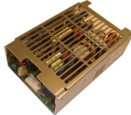
U-Chassis with Vented Top Cover
