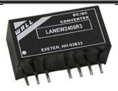
The LANEW3 Series offers 3 watts of output power from a 0.86 x 0.36 x 0.44 inch package without derating up to 71°C. The LANEW3 Series has a 2:1 wide input voltage range of 4.5-9, 9-18, 18-36 and 36-75VDC, it features 1600VDC I/O isolation, remote on/off, and short-circuit protection. All models are ideally suited for telecommunications, mobile telecom, test equipment, and industrial applications. For 3000VDC I/O isolation see the LANEW3 "H" Series.
