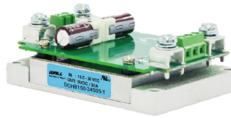
Terminal Block ("T" Suffix)
