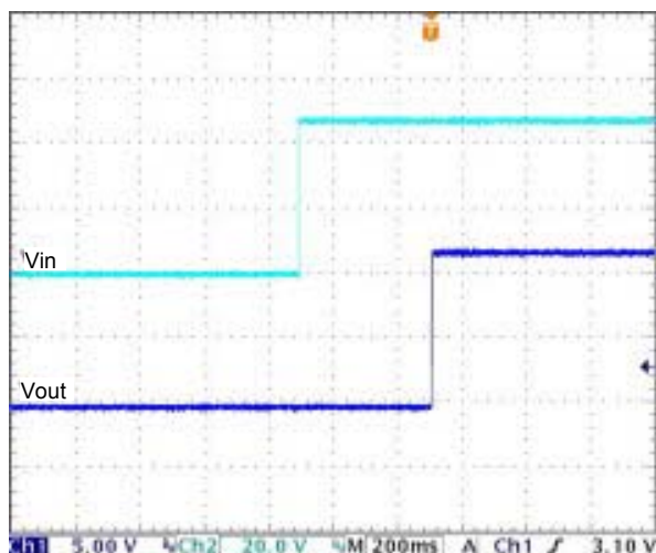
Graph 7: Typical Input Start-Up and Output Rise Characteristic (Nominal Vin and Full Load)
